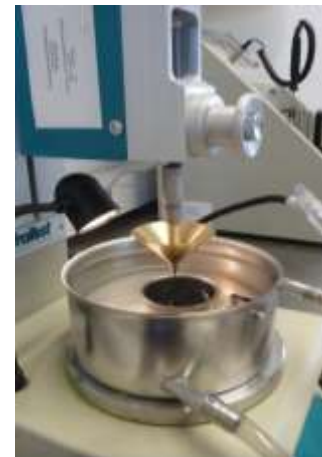
Cone penetration PN-EN 13880-2
